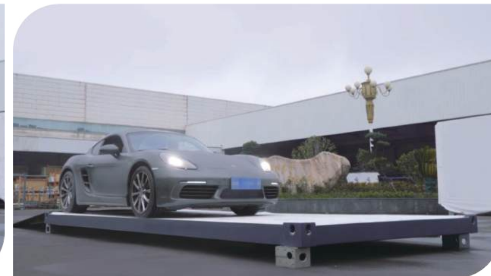
Container Roof 1.5T Load-bearing Test
