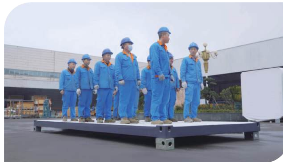
Container Roof 0.75T Load-bearing Test
